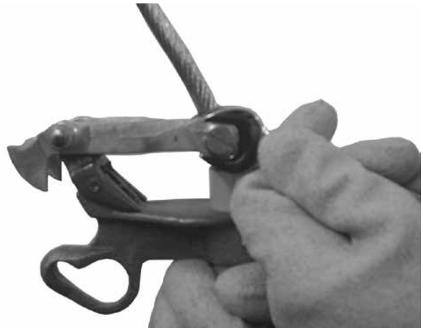
Figure 12. Secure fuse link leader..
