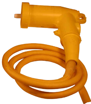
Figure 5. Grounding elbow is molded of bright yellow EPDM rubber for easy identification. Six-foot flexible copper, 600 volt insulated cable is available in 1/0 or 2/0. Elbow is fully rated for fault close to ensure operator safety.
