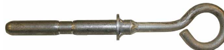
Figure 9. Test probe has an eye for easy hotstick handling. It allows electrical access to the bushing contacts so that circuit condition can be confirmed using appropriate test equipment. It should not be used for grounding because it has no fault-close rating.
