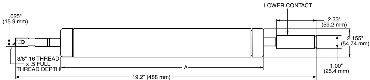
Figure 3. Dimensional information for single 2" diameter 8.3 kV and 15 kV E-rated and MSLE version ELSG fuses.
