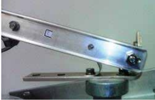
Figure 1. Optional 150D positive latch.
