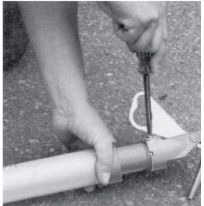
Figure 9. Hook open-fuse cutout pulling.
