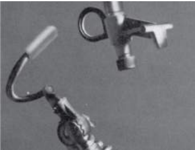
Figure 4. Hook open-fuse cutout pulling.
