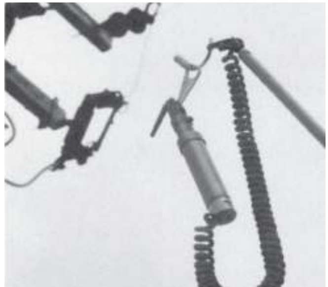
Figure 6. Removal of NX fault guard tool.
