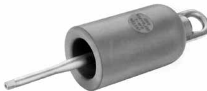
Figure 6. Catalog Number OT625. The Operating and Testing Tool is used with a hotstick to test for circuit de-energization and to install and remove a 25 kV Class LRTP equipped connector from an apparatus tap. The standard tool is equipped with a molded EPDM rubber cap to ensure tool seating and gripping of the T-OP II connector.
