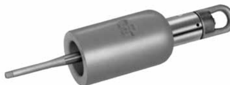
Figure 8. Catalog Number OTTQ625. The combination Operating and Test/Torque Tool is used with a hotstick to test for circuit de-energization and to install and remove a 25 kV Class LRTP equipped connector from an apparatus tap. The standard tool is equipped with a molded EPDM rubber cap and torque limiter to allow proper tool seating and gripping of the T-OP II connector. It also ensures that the connector has been properly torqued into the mating bushing.
