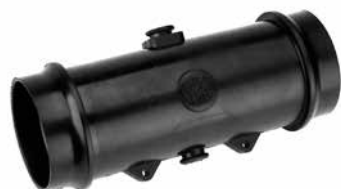
Figure 3. Catalog Number DBE625. The twin 600 A interfaces of the bushing extender allow installation on standard de-energized 600 A deadbreak interfaces for coupling loadbreak reducing tap plugs, connecting plugs and apparatus bushings. When assembled to mating apparatus, the bushing extender provides a completely submersible, fully shielded unit that meets the requirements of IEEE Std 386™-2006 standard. Refer to Service Information Section S600-59-3 for additional installation instructions.
