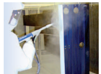
Electrostatic powder coating Applied to all surfaces prior to assembly.
