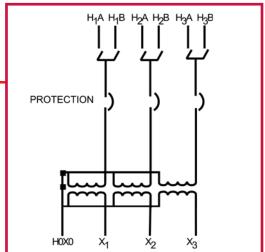
Schematic B: Three-phase VFI transformer with loop protection
