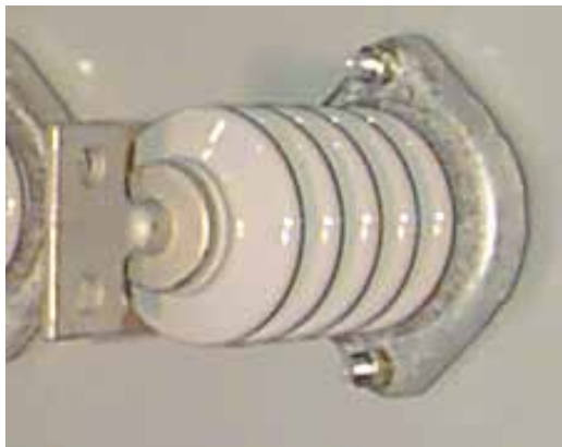
Figure 7. High voltage bushing.
