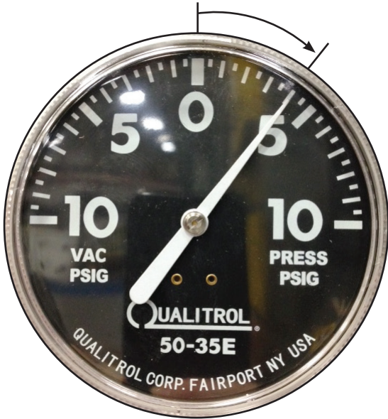
Figure 1. Ideal Operating Range (0 to +4 psig) for Transformer Pressure.
