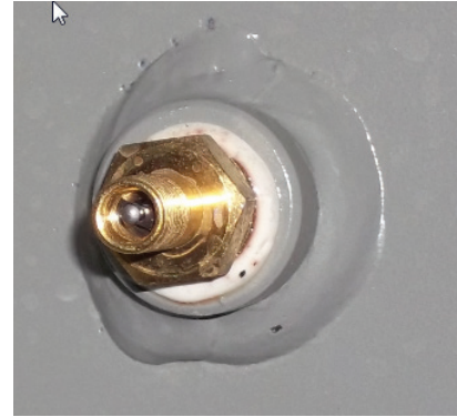
Figure 5. Add nitrogen via the Schrader valve.
