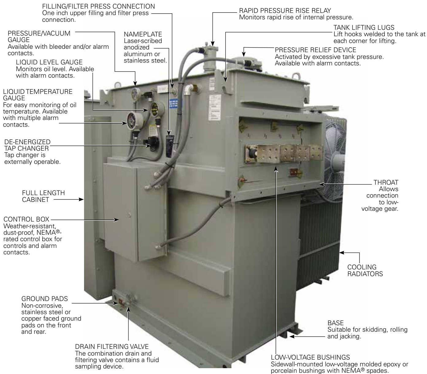
Figure 1. PEAK substation transformer with standard features and optional accessories.
