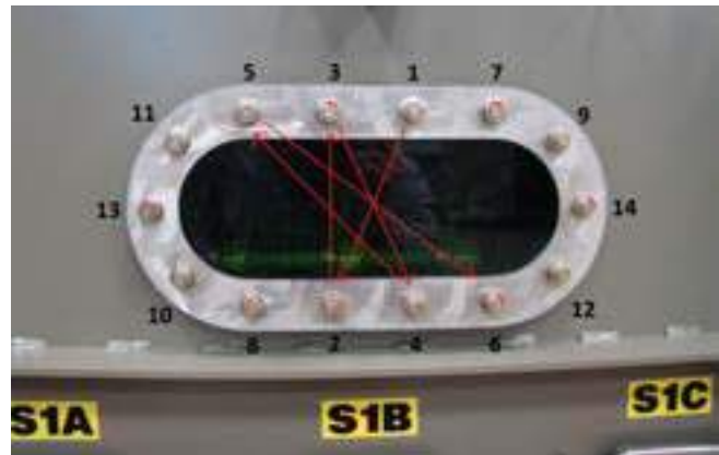
Figure 3. Mount the gasket, window, steel ring, and hardware.
