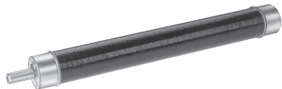
Figure 4. ELSG fuses provide current-limiting protection in series with an expulsion fuse, mounted in the wet-well holder.
