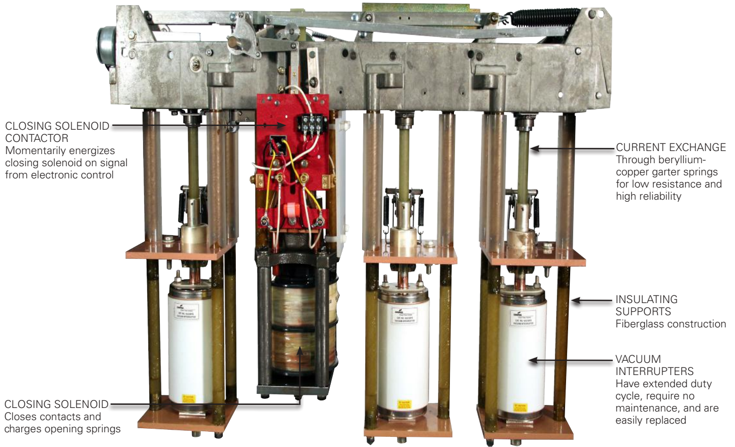
Figure 3. View of untanked PWE recloser shown from closing contactor side (low-voltage closing accessory shown). Construction of Type PWVE is similar
