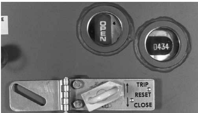
Figure 15. CI switch trip-reset lever
