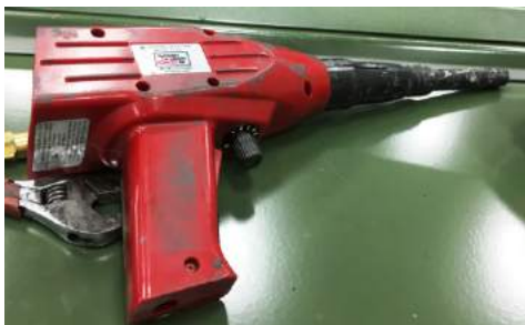
Figure 15. EFI Microsonic Detector Model EI-701 leak detector
