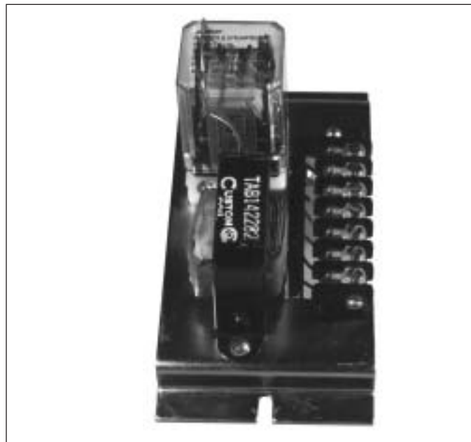
Figure 7-4. SCADA relay and terminal block
