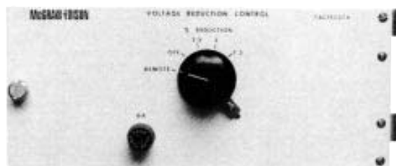
Figure 5-2. Voltage reduction control.
