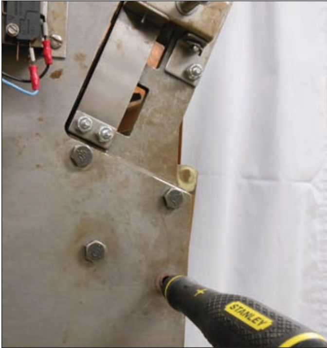
Figure 5. Inserting screwdriver to hold shim.
