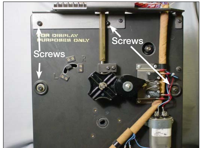
Figure 14. Drive Panel and Contact Panel Fastening.
