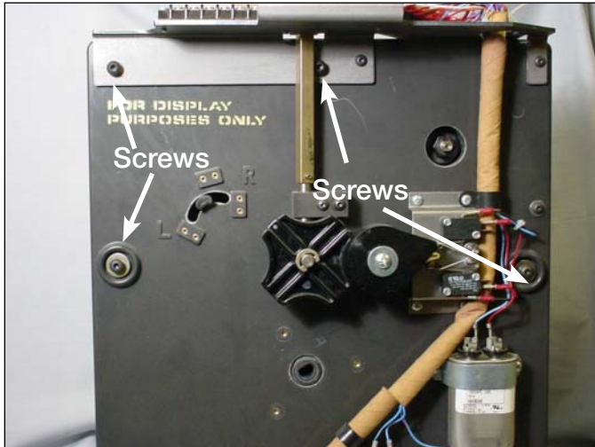
Figure 36. Panel Assembly Fastening.
