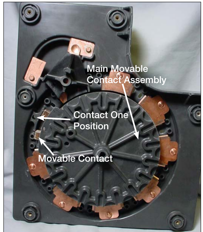
Figure 19. Positioning of Movable Contacts.
