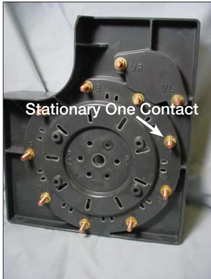
Figure 16. Removal of Stationary Contact.
