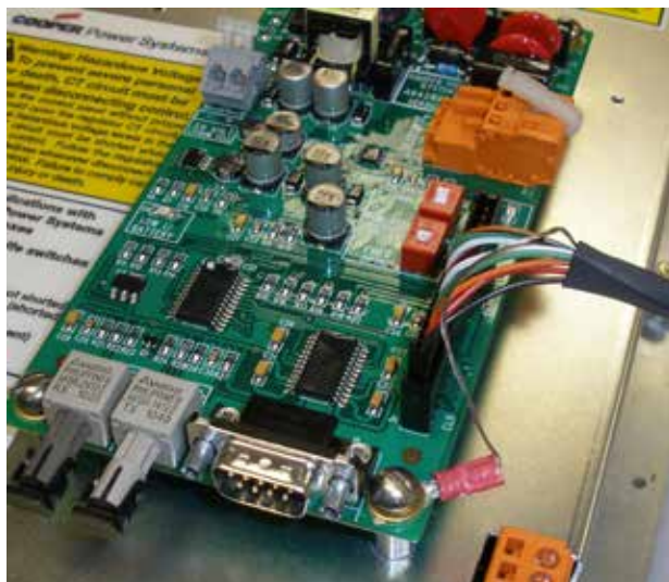
Figure 4. Connecting interface cable to module.
