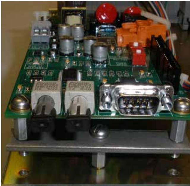
Figure 12. Communications module mounted using alternate method.
