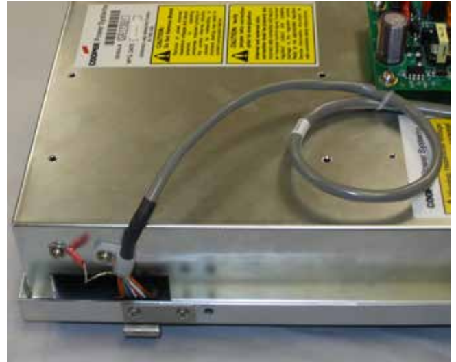
Figure 5. Connecting interface cable to CL-6B control panel.
