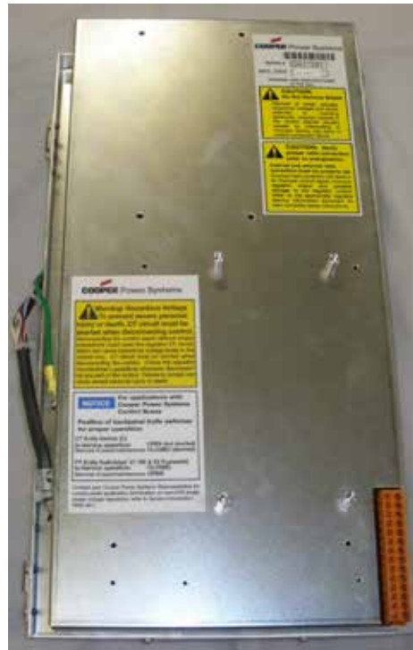
Figure 2. Stand-off studs on control panel.
