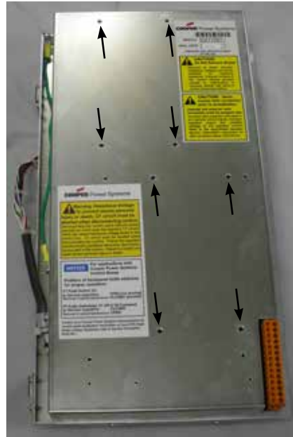
Figure 1. Communications module mounting locations, rear of CL-6B control panel.
