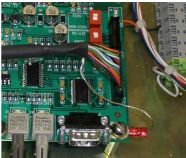
Figure 13. Connecting interface cable to module.
