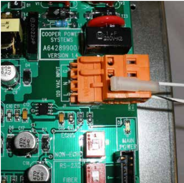
Figure 6. Connecting power to communications module.
