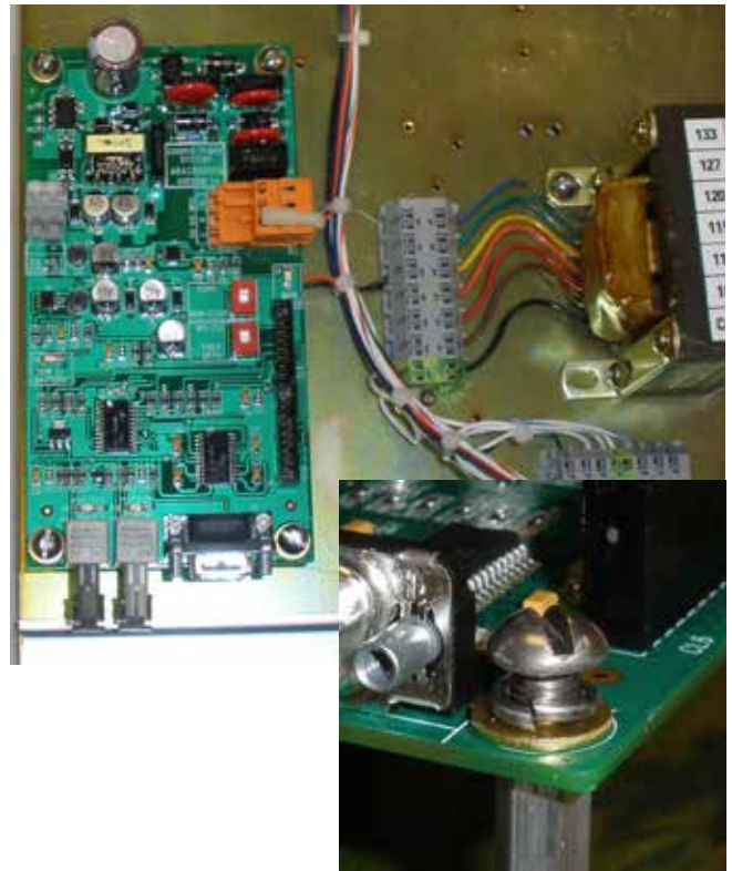
Figure 10. Module mounted on control box back panel.
