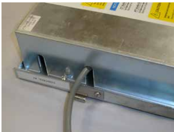
Figure 16. Routing interface cable on CL-5 control panel.
