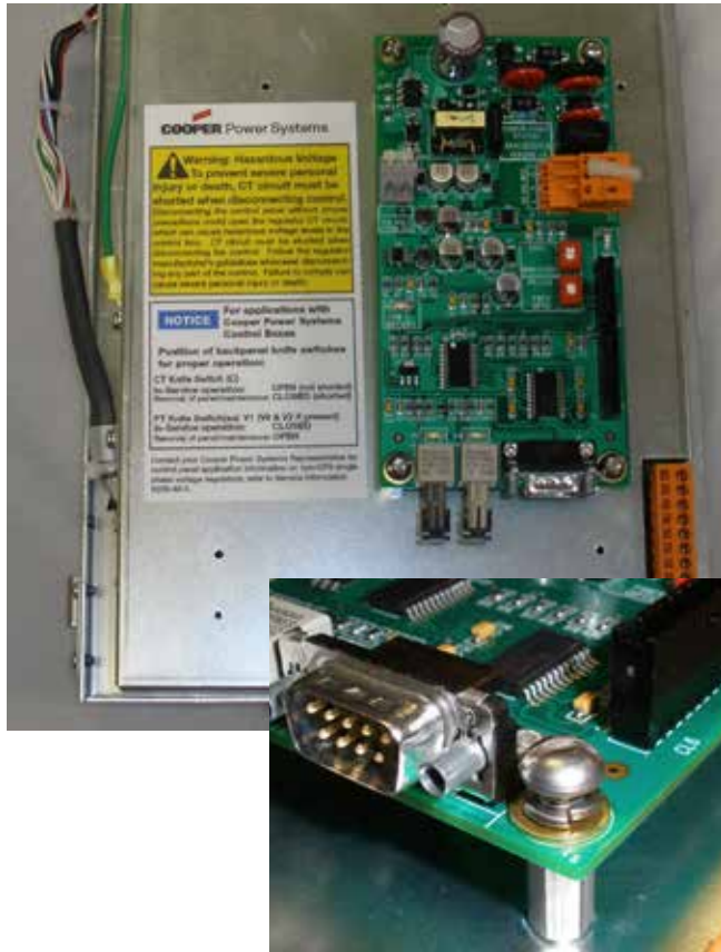
Figure 3. Module mounted on rear of CL-6B control panel.
