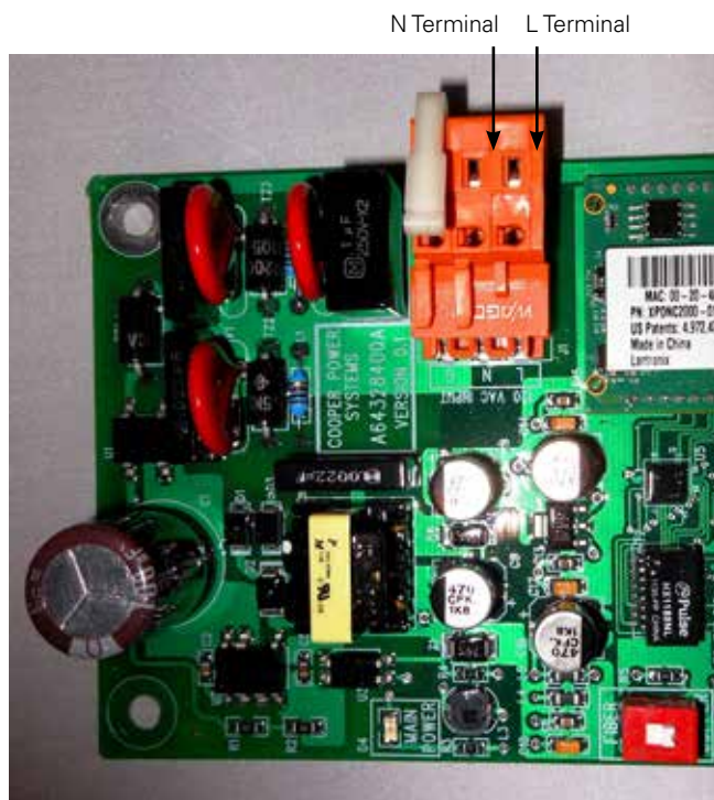
Figure 3. Connecting power to module.
