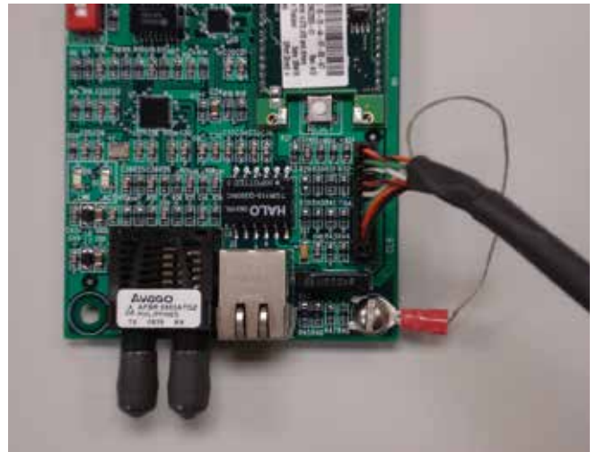
Figure 5. Connecting interface cable to module.
