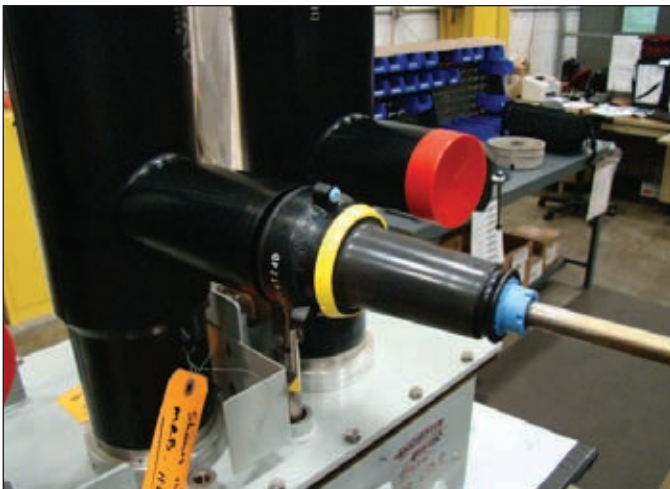
Figure 12. Torque BT-TAP or deadbreak connector plug.
