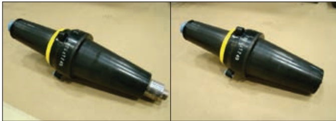
Figure 2. BLRTP with adapter (left) and without adapter (right).
