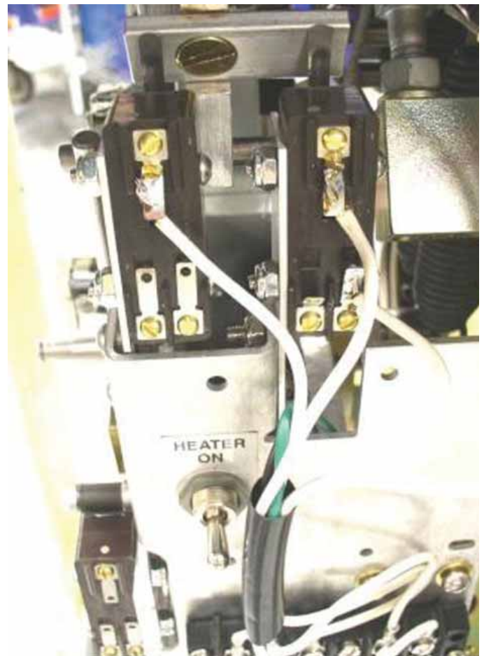
Figure 39. Positioning microswitch mounting plate.
