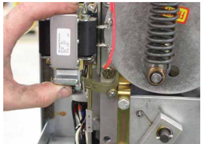
Figure 47. Cranking unit until lever snaps against latch.
