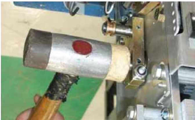
Figure 11. Tapping shaft end.
