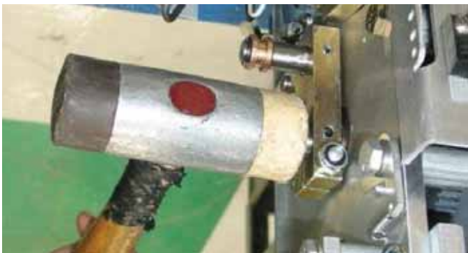
Figure 33. Tapping shaft end.
