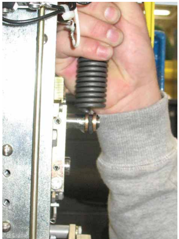
Figure 7. Removing spring from bronze bushing.
