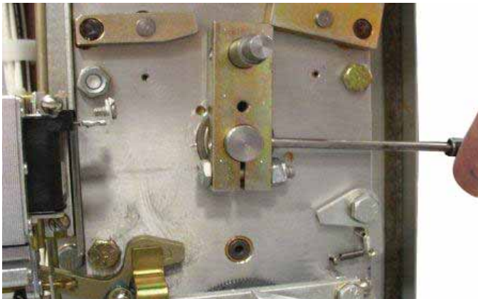
Figure 32. Removing roll pin.
