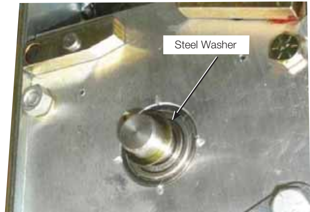
Figure 12. Removing shaft and washer.
