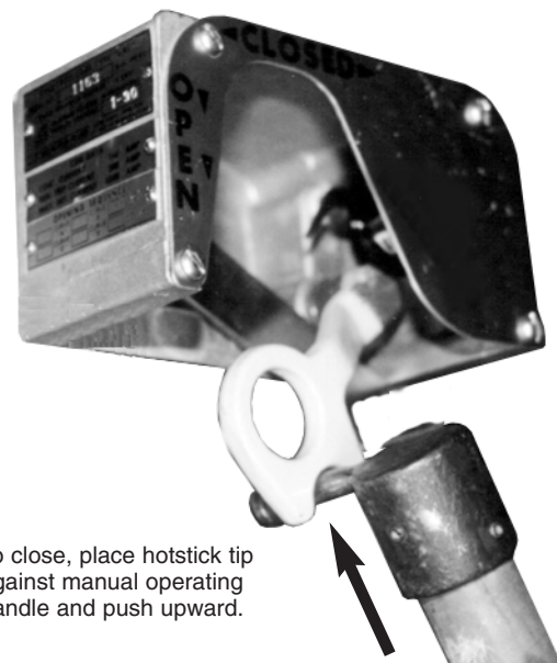
Figure 5. Correct placement of the hotstick to close the switch.
