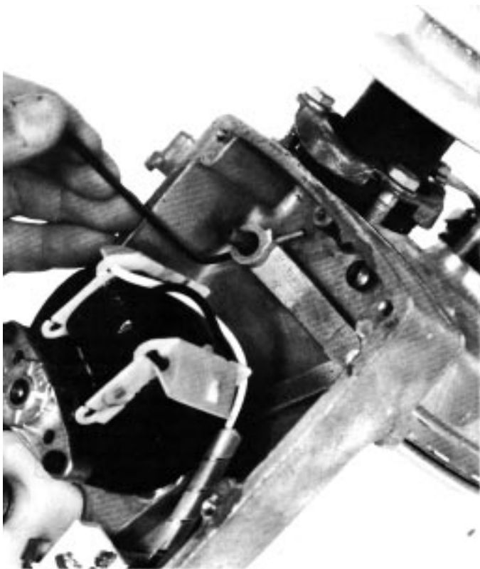
Figure 20. Removing straight pin with allen wrench.
