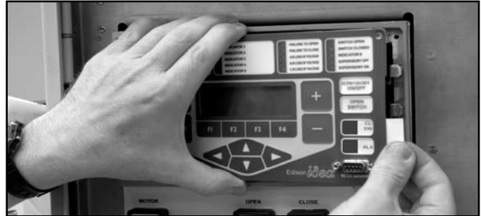
Figure 24. Removal of inserts from front operation panel of iMC switch control.
