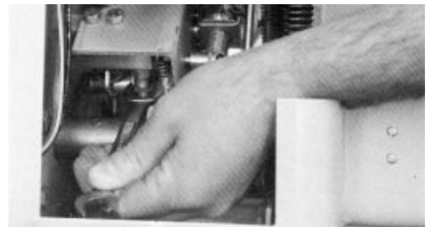
Figure 18. Setting stop bolt.
