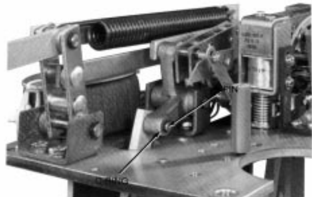
Figure 17. Contact box replacement.
