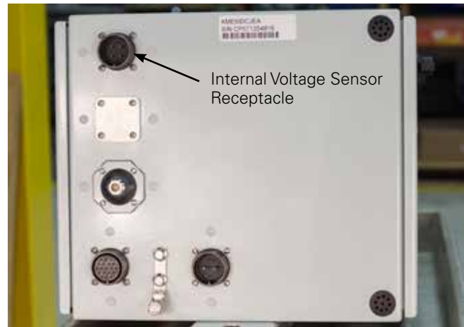
Figure 33. iDC control internal voltage sensor receptacle.
