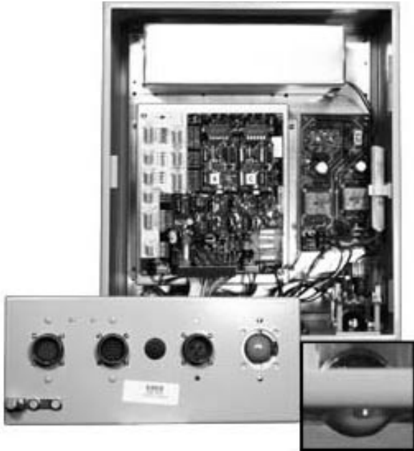
Figure 1. NOVA 1 Recloser Control with close-up view of cable receptacles and ball-target lockout indicator.
