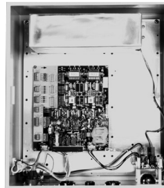
Figure 1. Kyle ® NOVA 1 single-phase, electronically controlled recloser and control.
