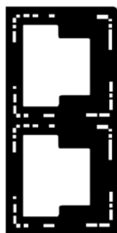
Figure 2. End view of battery connector – 24 Volt battery configuration.
