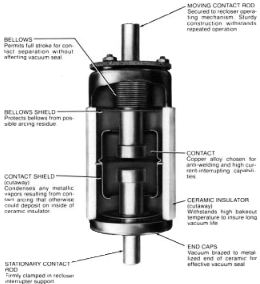
Figure 15. Cutaway of typical vacuum interrupter.
