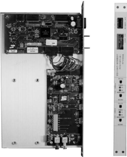
Figure 1. Fiber-Optic/RS-232 serial communications accessory circuit board side and front view.
