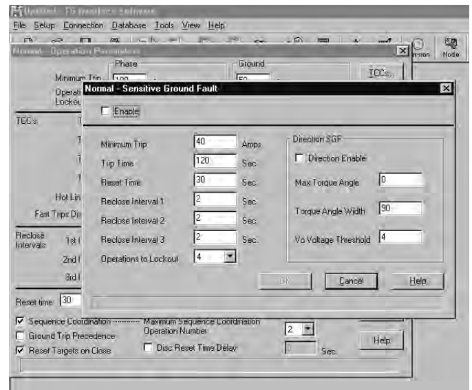
Figure 17. Directional SGF/SEF configuration screen.
