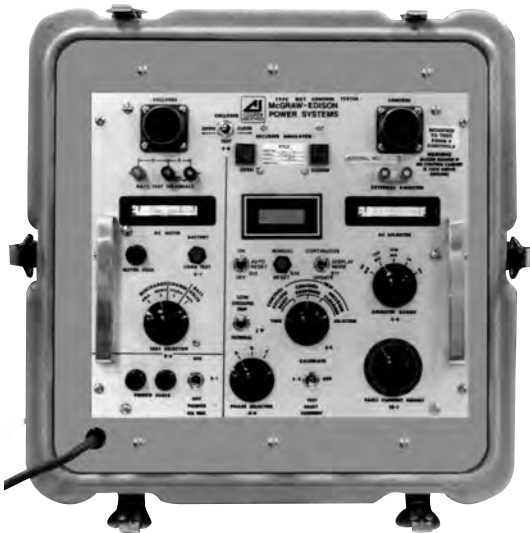
Figure 41. Kyle® Type MET electronic recloser control tester.
