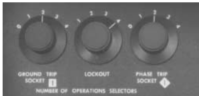
Figure 8. Ground-Trip, Lockout, and Phase-Trip Operation Selectors.
