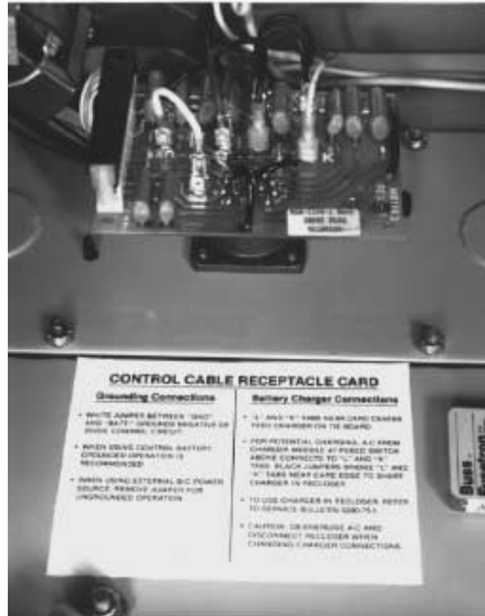
Figure 21. To use Charger in Recloser, Jumpers on Control Cable Receptacle Card must be changed.
