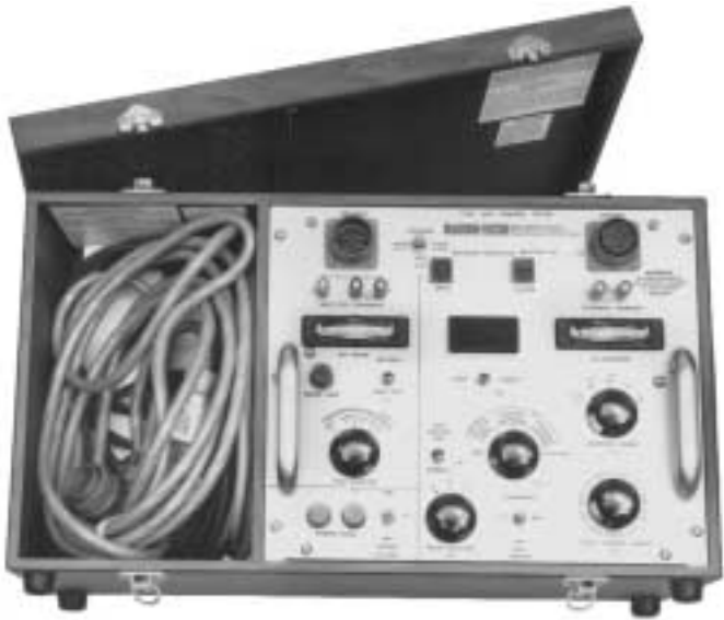
Figure 23. Kyle Type MET Electronic Recloser Control Tester.
