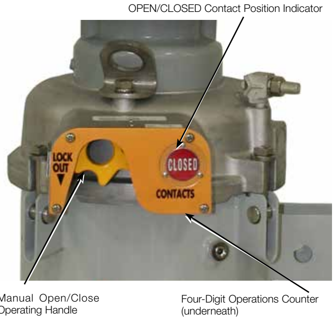
Figure 18. SPEAR single-phase recloser operating lever and indicators.
