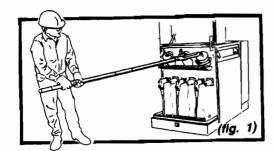
**CAUTION:** Remove and park all load side separable connectors and install insulated protective caps on tap bushing before installing or removing fuse. Fuse IS NOT a loadbreak device.
