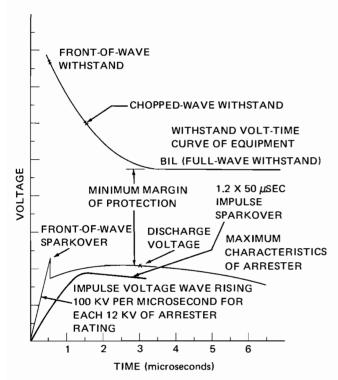
Typical volt-time curve showing arrester characteristics compared with equipment insulation withstand characteristics.
