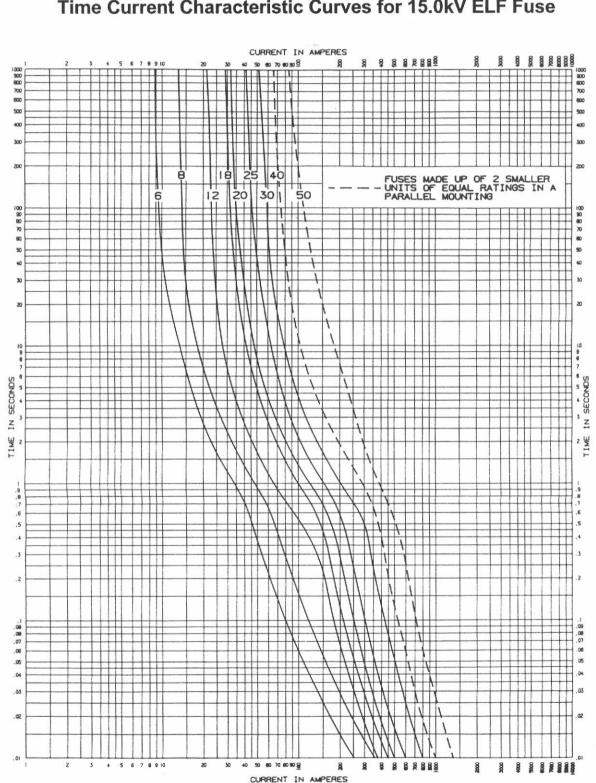
MINIMUM MELT Time Current Characteristic Curves for 15.0kV ELF Fuse
