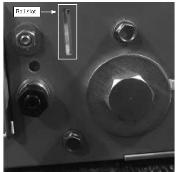
Figure 22. Outside view of cassette side sheet drill template secured to MDN cassette
