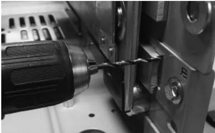
Figure 19. Drilling the top edge of template
