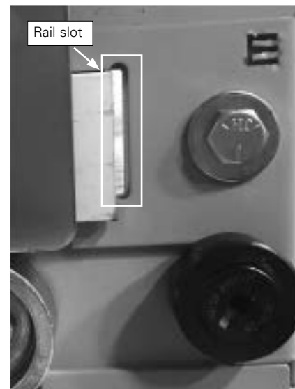
Figure 21. Inside view of cassette side sheet drill template secured to MDN cassette
