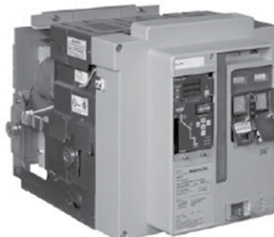
Magnum MDSL Current Limiting Power Circuit Breakers have integral current limiters to provide interrupting ratings of 200 kA at 600 Vac.
