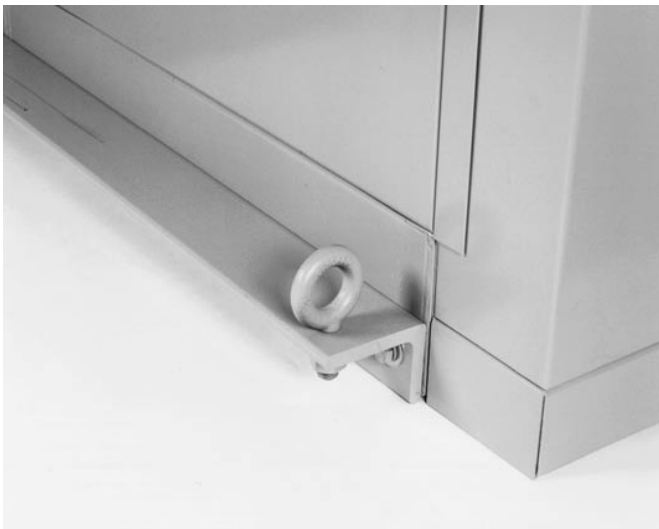
Figure 2. Figure 2 Lifting Angle in Place As Received Prior to Reversing for Securing to Foundation.
