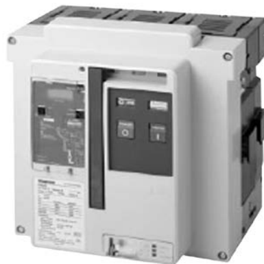
Magnum MDSX Current Limiting Power Circuit Breakers have fast opening contacts to provide interrupting ratings up to 200 kA at 480 Vac without current limiters.
