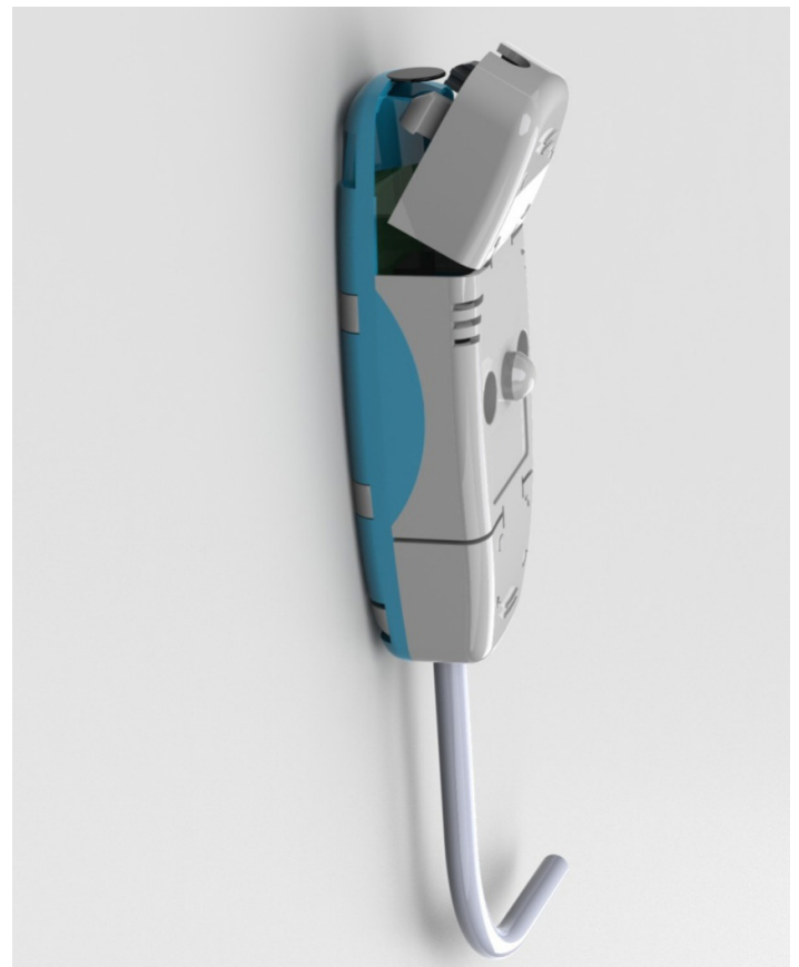
Figure 5. EAFR-01 point sensor mounted to the compartment wall.
