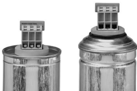
Bulged capacitor cell top provides easy visual indication of pressure interrupter operation
