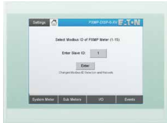
Figure 6. Changing the Modbus ID.
